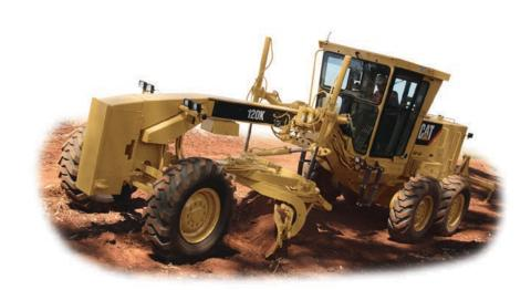
The 120K optimizes your investment by delivering maximum productivity and durability. The Cat C7 engine, direct-drive power shift transmission and load-sensing hydraulics work together to ensure the power and precision to get the job done.
